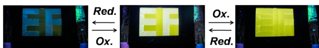
Figure 6. Photographs are the image of the reversible FL switching cell, at given potential.
